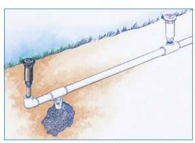
Automatic Drain Valve Installation for Freezing Climates: Locate the drain valves at the low points in each zone.
