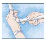
PVC: 2. Slip pipe into fitting and wipe off excess solvent.
