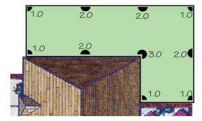
AREA C = 16 GPM PGJ MID-RANGE ROTORS
