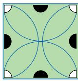
**Step 2**Add sprinklers along the sides if necessary.
